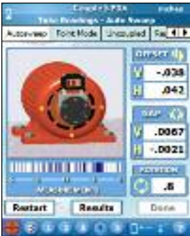
Take Readings – 4 data taking modes for maximum flexibility and ease of use: Autosweep™ Mode, Point Mode, Uncoupled Mode or Clock Mode.
